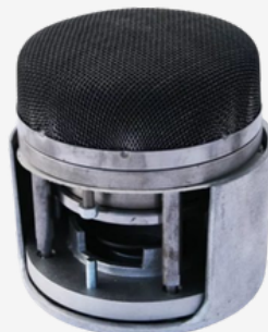
CRANKCASE EXPLOSION RELIEF VALVE
