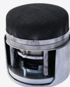
CRANKCASE EXPLOSION RELIEF VALVE
