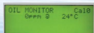
The backlit 4-line display provides easy menu driven commands for set-up, calibration, and diagnostics.
