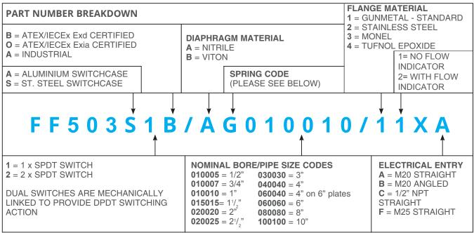
Spring code: This will be designated by our Engineer upon calculating the most applicable orifice ratio dependent on the pipe size, normal flow and alarm flow required for your specific application. These calculations will give a figure in "HG and the spring codes cover specific ranges.
