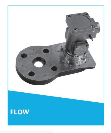
Each instrument can be provided with one of seven standard orifice ratios which enables a wide range of flow rates to be accommodated. When using fluids other than fresh water these values will of course alter. It should be also noted that the head loss values are those occurring immediately across the orifice and that up to 50% of this head loss can be recovered by providing at least ten diameters of straight plain pipe either side of flow switch.
