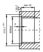
Fig.5b. Socket for T connection
