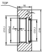
Fig.5c. Weldable fitting ring for T connection Sealing: teflon Order code Socket T
