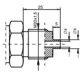
Fig.3a. M connection with M20x1.5 thread
