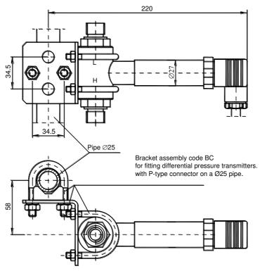
Figure 11. Example: how to install the PYRD-28.
