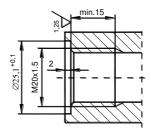
Fig.4b. Socket for P connection
