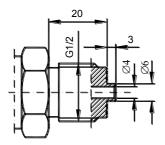
Fig.6a. GB connection with G1/2" thread
