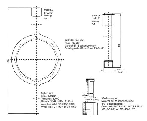
Figure 15. Additional equipment for fitting of pressure transmitters.
