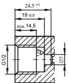
Fig.6b. Socket for GB connection.
