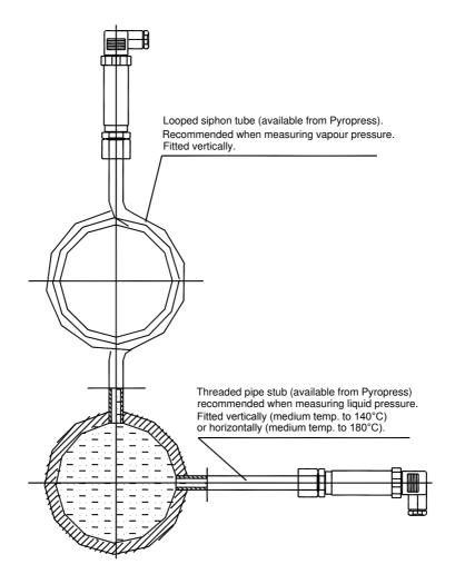
Figure 14. Possible methods of isolating the transmitter from high temperatures
