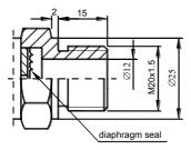
Fig.4a. P connection with M20x1.5 thread
