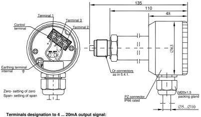
Terminal 1 - Supply "+" (plus) Terminal 2 - Supply "-" (minus) Terminal 3 - TEST\_SIGNAL
