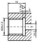
Fig.3b. Socket for M connection.
