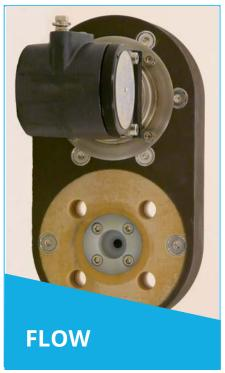
Each instrument can be provided with one of seven standard orifice ratios which enables a wide range of flow rates to be accommodated. When using fluids other than fresh water these values will of course alter. It should be also noted that the head loss values are those occurring immediately across the orifice and that up to 50% of this head loss can be recovered by providing at least ten diameters of straight plain pipe either side of the flow switch.
