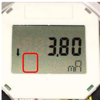
Figure 8: Mode 1 (without a digit) Measurement mode before calibration (a value differing from 4.00 mA is shown)
