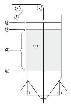
Install a weigh bin, (bin or silo equipped to provide a 4 to 20 mA output proportional to weight), preceding the material infeed.
