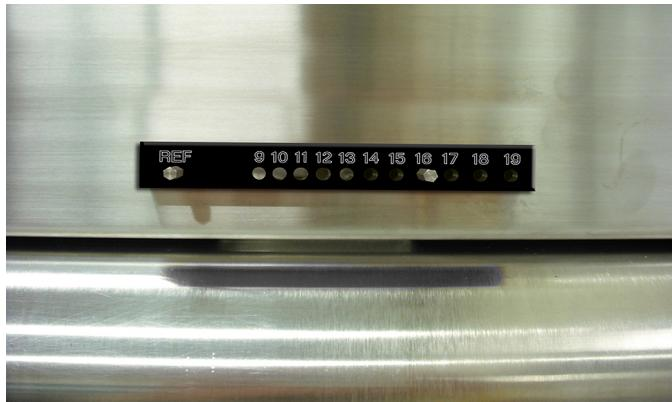
Figure B-38 Spacer bar
