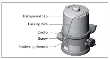
Fig. 4: Installation locking wire
