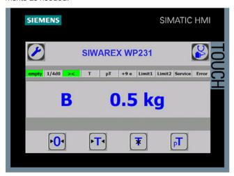
In addition to the configuration package, a fully-featured SIWAREX WP231 "Ready for use" software is also available free-of-charge. It shows beginners how to integrate the module in a TIA Portal program and offers a basis for application programming. This allows you to connect the scale application very easily to an operator panel either connected to the SIMATIC CPU or connected directly to the SIWAREX WP231.
