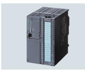
The SIWAREX FTC (Flexible Technology for Continuous Weighing) is a versatile and flexible weighing module for belt scales, loss-in-weight feeders and solids flowmeters. It can also be used to record weights and measure force.
