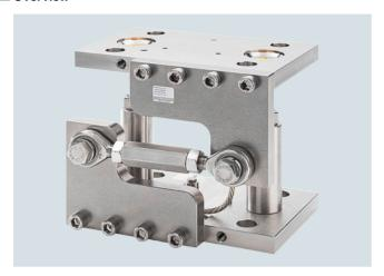
The self-centering mounting unit for SIWAREX WL270 CP-S SA load cells is particularly suitable for implementation in container, platform, vehicle and roller table scales. The guide elements prevent containers, for example, from moving sideways due to an external lateral force. The guide elements can be mounted on one or both sides of the compact mounting unit.
