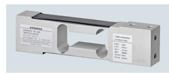
The load cell is suitable for small platform scales with one load cell and a max. platform size 400 x 400 mm (15.75 x 15.75 inch) as well as for use in medium accuracy weighing machines of Class III with a max. scale verification intervals  $n_{max} = 3000d$ .
