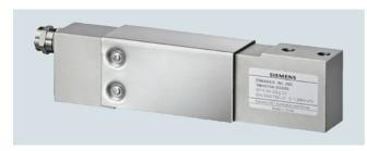
The load cell is suitable for small to medium platform scales with one load cell and platform size up to 400 x 400 mm (15.75 x 15.75 inch) as well as for use in medium accuracy weighing machines of Class III with a max. division  $n_{\text{max}} = 3\ 000\text{d}.$
