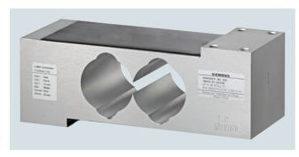
The load cell is suitable for small to medium platform scales with one load cell and platform size up to 600 x 600 mm (23.62 x 23.62 inch) as well as for use in medium accuracy weighing machines of Class III with a max. division  $n_{\text{max}} = 3\ 000\text{d}.$
