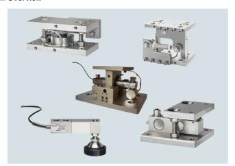
The use of SIWAREX WL200 installation accessories avoids incorrect loading such as eccentric load introduction, torsion torques etc. on the load cells. enables full exploitation of the measuring accuracy of the load cells.
