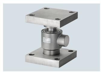
In combination with a pressure piece set and adapter plate, the SIWAREX WL270 CP-S SA load cell produces a self-aligning bearing. This unit is particularly suitable for installation in hopper scales, bin weighing equipment and vehicle scales.
