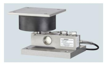
The base plate and the elastomer bearing form a self-centering bearing unit together with the load cells of the SIWAREX WL230 SB-S SA series. It suppresses oscillations and shocks to a certain extent.
