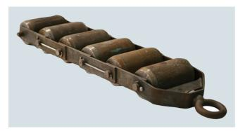
Roller test chains are used for belt scale calibration when material tests are not practical. All test chains are bushed. Minimum length is 4 feet (1.2 m).
