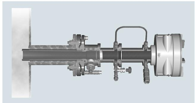
Sensor configuration with high purging on the process side, with 6 mm joint for use with steam, and with N<sub>2</sub> purging on the sensor side
