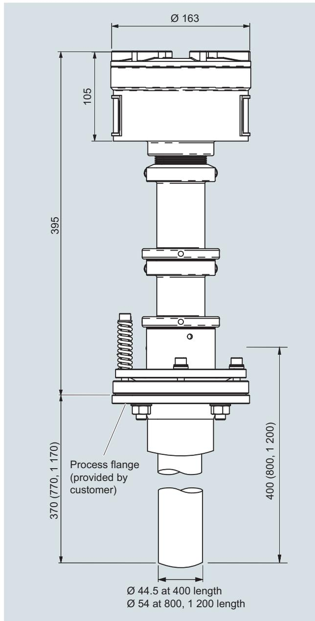
Cross-duct sensor CD 6, increased purging (instrument air), version according to Order No. 7MB6122-\*\*E1\*-0\*\*\*, dimensions in mm
