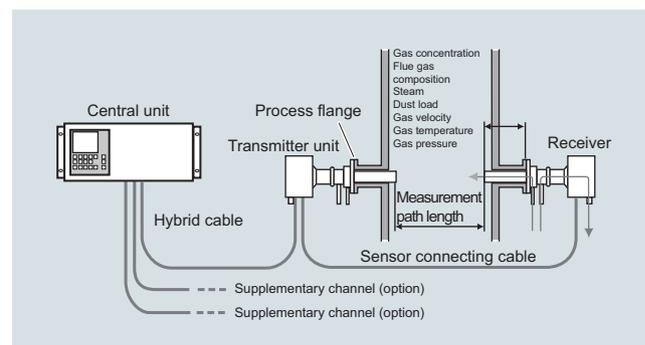
Typical transmitted light setup of LDS 6, in-situ
