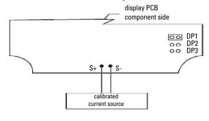
The display PCB may be removed from the enclosure for bench calibration. Loop jumper must be installed on input signal PCB to maintain loop. Refer to *Servicing display PCB outside the loop* on page 9.
