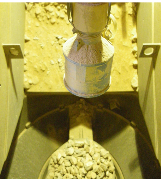
An Echomax transducer measuring the level in a crusher.
