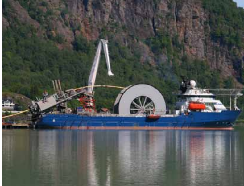
Cable- and pipeline-laying machinery, like that on the stern of the ship, above, use weighing technology to monitor forces created by the moving cable or pipeline.
