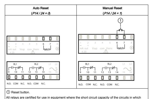
they are connected is limited by fuses having ratings not exceeding the rating of the relays.
