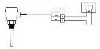
$R_{max} = (V_{supply} - 12 V)/20 mA$
