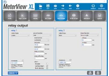
▲ The Relay Output window is used to assign a specific task to the 2 relays such as alarm, sample, timer, stopwatch, or off. A custom message that will flash every 10 seconds can also be added.
