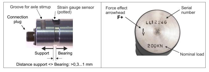
Note: For a measurement with highest possible accuracy, it is necessary to sufficiently lubricate all movable parts (e.g. fairleads, rope guides) inside the entire installation.
