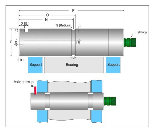
LASTMB load measuring pins are manufactured customizable, every dimension is possible. Electrical connection is realized either with a plug or with a cable connection.
