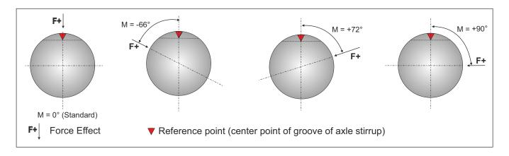
The standard version of the LASTMB load measuring pin assumes the force will be applied vertical to the reference point (center point of groove of axle stirrup). If local conditions make this impossible, please specify an angle of deviation.
