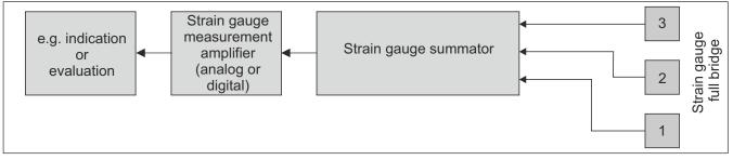
One installation consists of 3 load measuring pins with one strain gauge full bridge each. The three strain gauge sensors are connected together into one summator. The sum signal will be transferred onto a strain gauge amplifier. The next device downstream will further process the output-signal of the amplifier.
