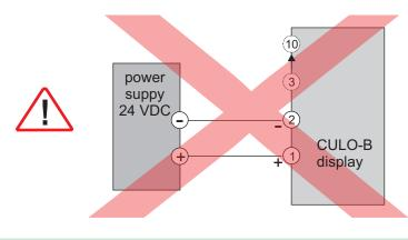
The input 0(4)...20 mA has to be operated with a mA-signal only. A direct connection to a voltage supply (eg 24 VDC) will destroy the indicator and the guarantee does not cover this.
