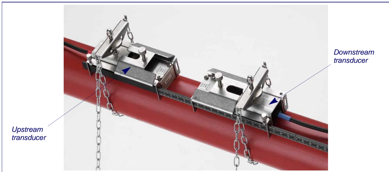
Figure 2.4 Completed transducer assembly
