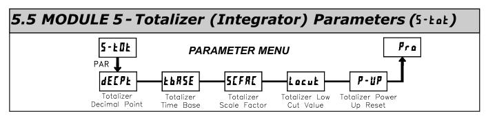
The signal totalizer (integrator) can be used to compute a time-temperature product. This can be used to provide a readout of temperature integration, useful in curing and sterilization applications. The second is through a user input or function key programmed for Batch (one time add on demand). If the Totalizer is not needed, its display can be locked-out and this module can be skipped during programming.
