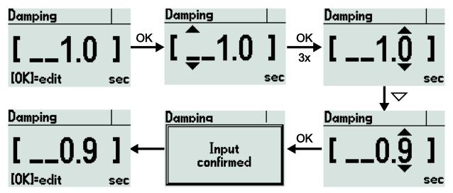
Figure 7: Procedure for setting a numeric value (e.g. from 1.0 to 0.9)
