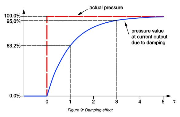
The damping affects the current output as well as the displayed pressure value.
