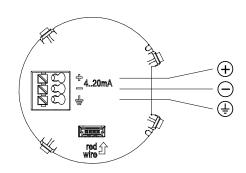
Figure 1: Options for the electrical connection
