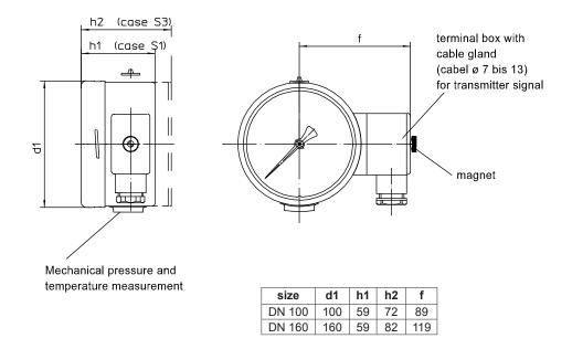
Electronical angle-of-rotation sensor with electrical zero setting (option) integrated in a safety pattern gauge EN 837-1 S1 and EN 837-1 S3
