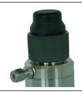
Once the storage cap has been removed, an orange sticker will be visible informing you not to remove the protection cap. This is because the sensor has already been checked and calibrated prior to shipping, and no sensor maintenance or membrane change is required prior to first use. However, this label must be removed.
