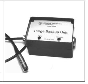
The 32605 purge backup unit is connected between the instrument and the sensor. The internal batteries are automatically charged through the sensor cable when the instrument is turned on.
