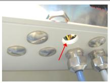
1. Select an unused opening nearest to the cable connection on the electronic board. Remove the screw and nut combination and set aside the screw for later use.
