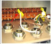
7. Connect the wires to the correct terminals.
