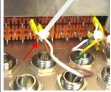
8. Secure the wires with a cable tie.
