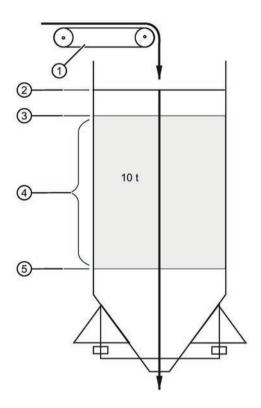
Install a weigh bin, (bin or silo equipped to provide a 4 to 20 mA output proportional to weight), preceding the material infeed.
