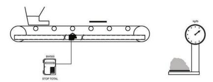
% span adjust = (BW500 - material sample weight) x 100/ material sample weight
