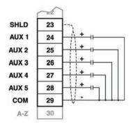
Customer dry contacts, or open collector transistor output supplied as required.
